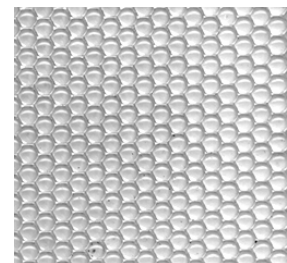
Figure 29 - enlarged fly's-eye lens [20]
